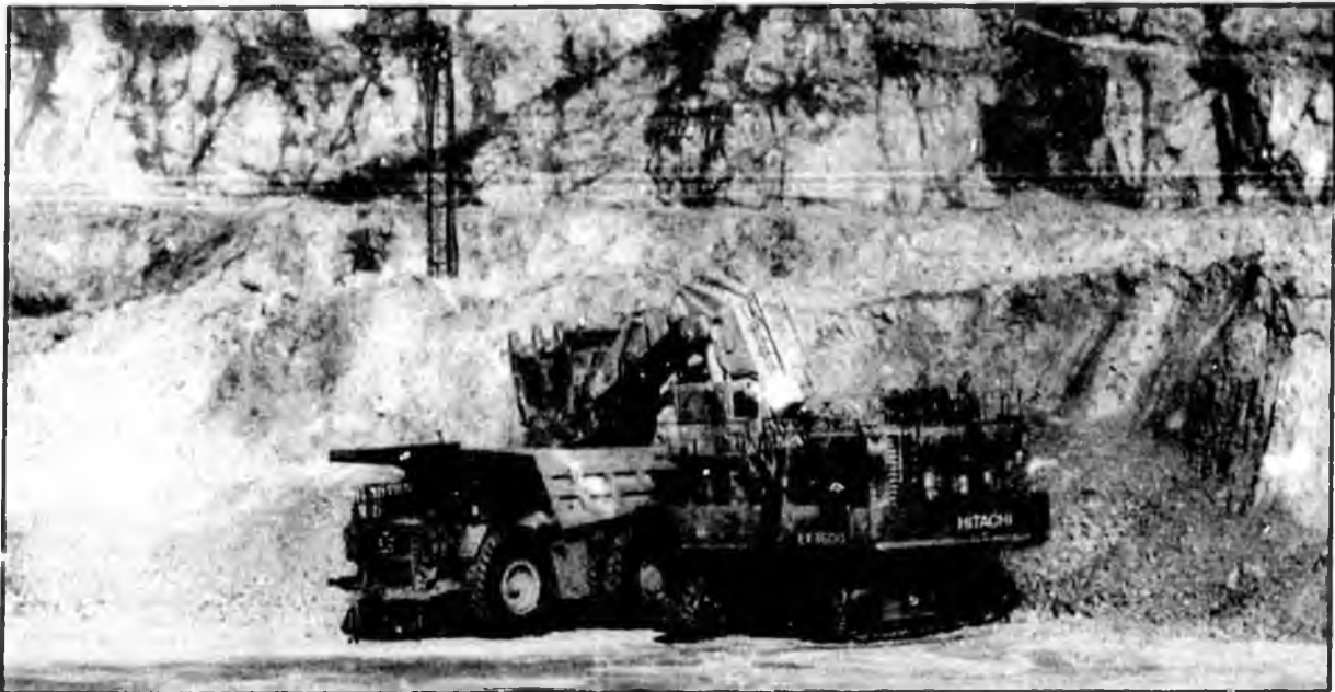
SH6 loads a haul truck with ore that will tip the scales at close to 200-tons.
