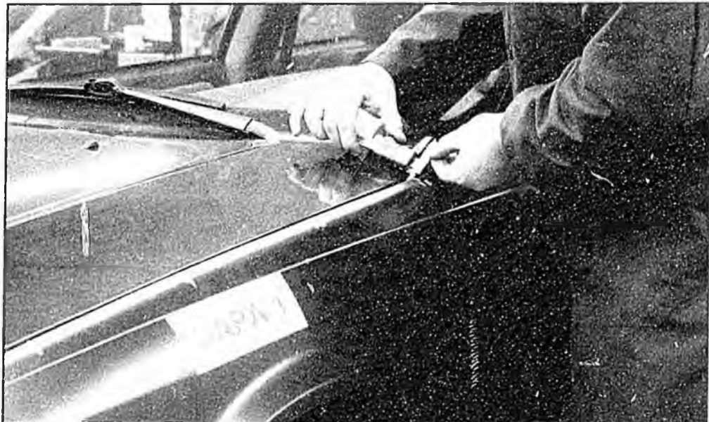
Checking gap during Vehicle Test Fit
