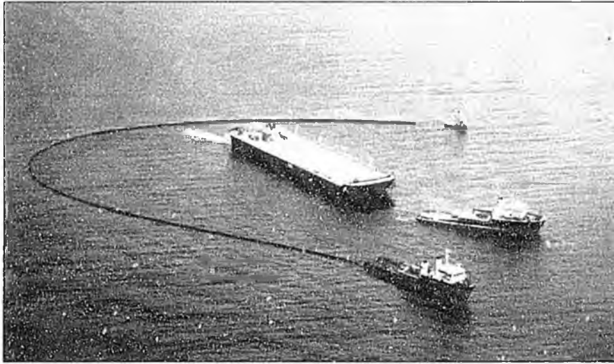
Practice—a tanker is surrounded by boom during a major spill drill.
