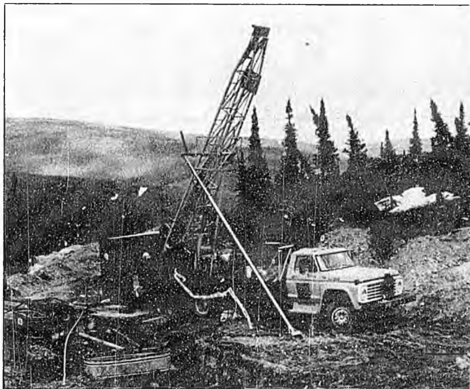
Figure 18. Drilling equipment at Fort Knox deposit near Fairbanks. Most of the drilling on the property in 1991 was condemnation drilling carried out so that future mining activity would not be compromised by the mine's infrastructure. (Photo by Fairbanks Gold Ltd.)
