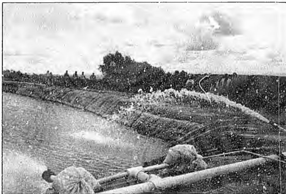
Figure 10. Inco Exploration and Technical Services Inc. neutralize cyanide at the heap leach project at the Ryan Lode on Ester Dome. (Photo by R.C. Swainbank)
