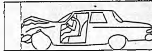
On impact, the car begins to crush and slow down. The person inside continues to move forward at the same speed the car was traveling. Within 1/10 of a second, the car has come to a stop, but the person is still moving forward.
