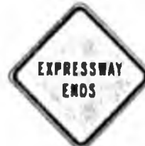
Pavement ahead is unfinished or barricaded. Slow down, leave expressway.
