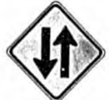
Warning of change from divided highway to two-way traffic ahead.
