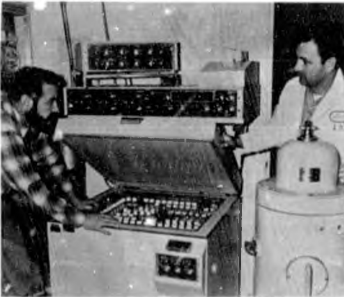
J. R. Luick (left) and D. F. Holleman (right) are shown discussing the liquid scintillation counter that is used to measure radioactive isotopes in various biological samples.
