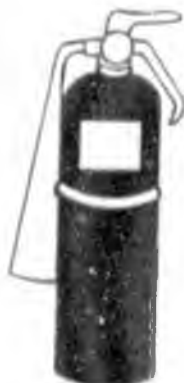
Freon Type Extinguisher
