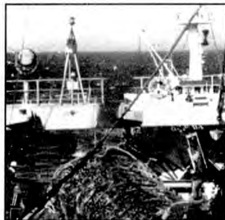
A factory trawler in the Bering Sea retrieving a codend filled with approximately 40 tons of pollock.
