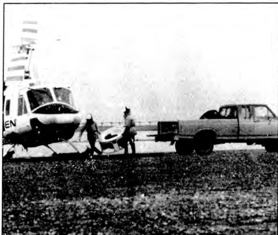
Komara 12K skimmer head is stowed on board a Bell 212 helicopter for remote river delta deployment
