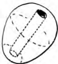
Marker or mooring buoy
