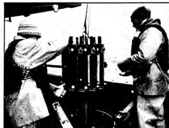
Institute of Marine Science technicians on board the R/V Alpha Helix collect Bering Sea water samples from the CTD rosette for shipboard and laboratory analysis. (Photo: Geoffrey Orth)
