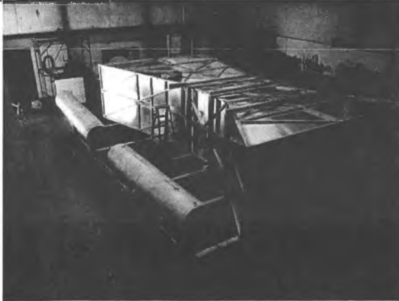
Assembled venturi box and ballasts
