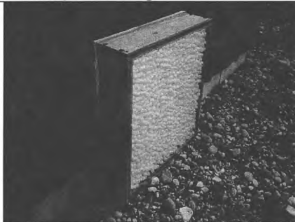
UV stability test of the EPS beads
