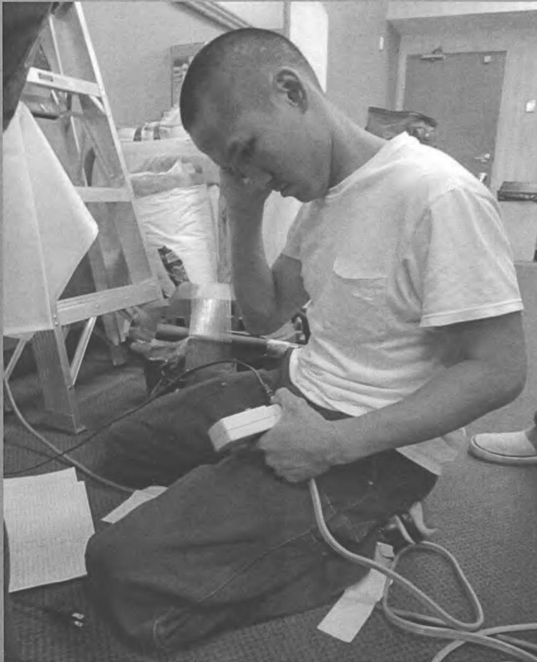
Crews Test Appliances with Kill-a-Watt Meters
