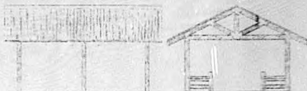
Pavilion sides left open, with no siding or windows.
