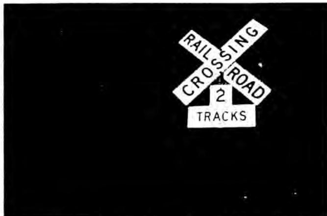
Experimental illumination material may make railroad crossbuck warning signs more visible during the dark night time hours.
