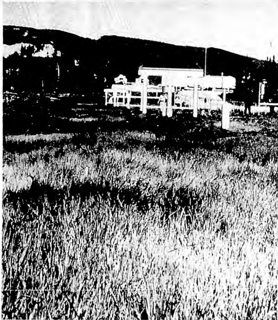
This field of grass was grown in six weeks by botanists at Arctic Gas' $3.5 million Arctic test facility at Sans Sault, NWT. A ditch had been dug to accommodate a stretch of 48-in. diameter pipe for testing purposes and then was covered and seeded to see how quickly and effectively a vegetative cover could be restored.
