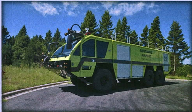
Gustavus Aircraft Rescue and Fire Fighting (ARFF) truck. Photo courtesy of Rosenbauer (manufacturer).
