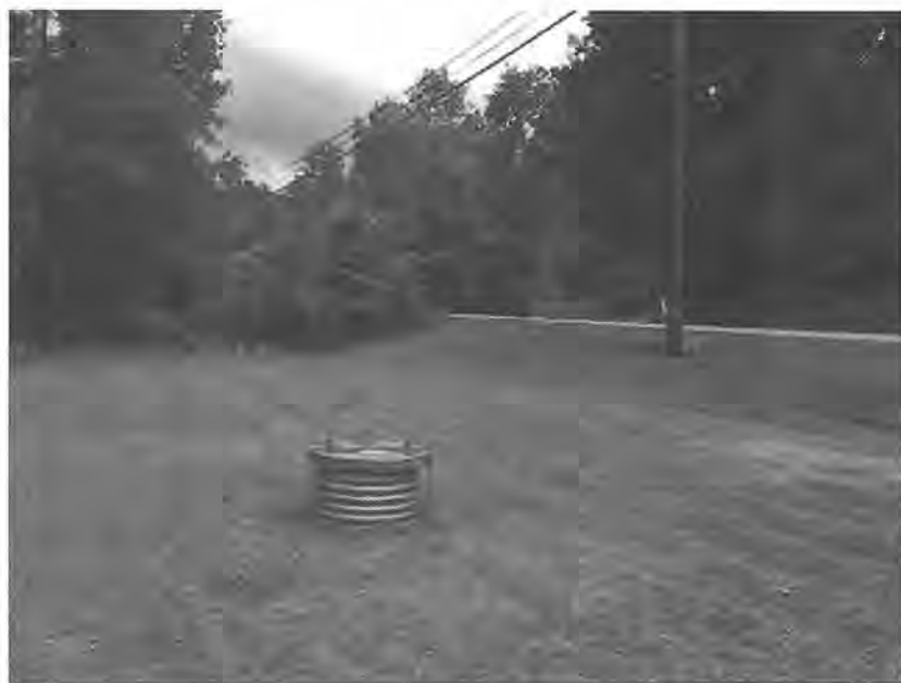
FIGURE 1—First scenario: pentachlorophenol-treated pole near contaminated well.
