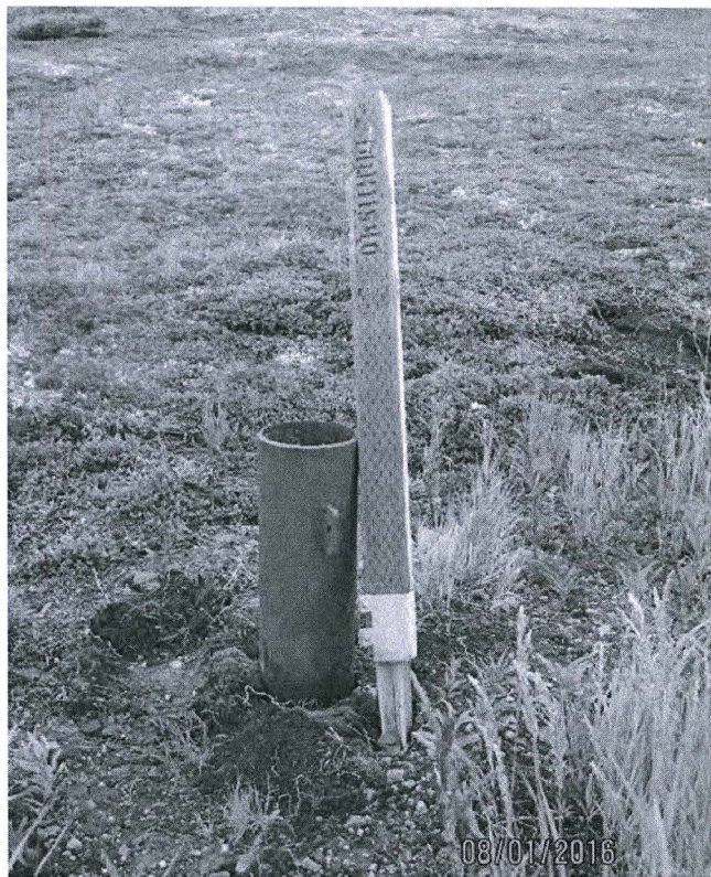
Figure 5: Steel drill casing at reclaimed drill site DDH 11540, drilled in 2011.
