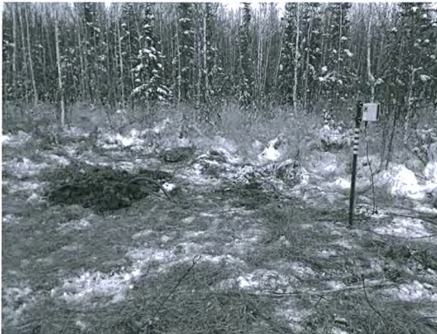
Photo 2: Example of a casing and a casing with temperature acquisition cable and fiberglass unistrut post with datalogger.
