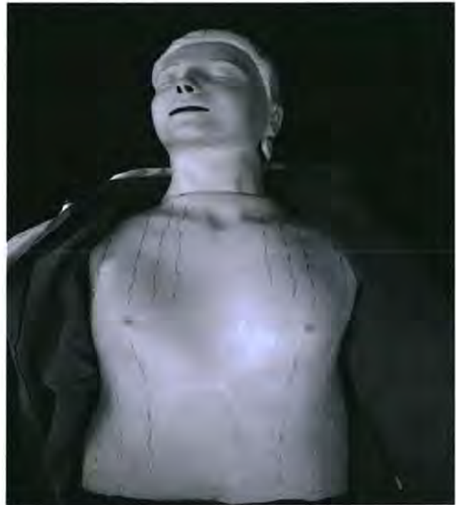
FIGURE 1. The manikin with wires stitched into the skin covering the right and left sides from the upper chest through the abdomen. The wires were attached inside the manikin to a rhythm simulator to provide the electrocardiographic (ECG) ventricular fibrillation (VF) signal. The wires allowed transmission of impedance and ECG signals to the electrode pads simulating a patient in VF.
