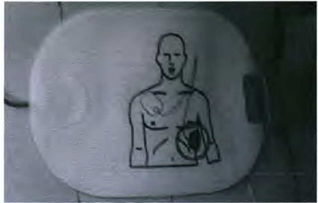
FIGURE 4. Icon for AED1 (one of the four automated external defibrillators studied) depicting the relative locations for both pads.
