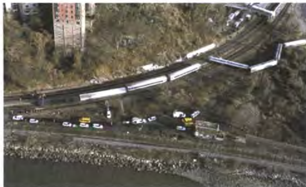
In 2013, a Metro North passenger train in Bronx, NY derailed when the engineer fell asleep going 82 MPH in a 30 MPH curve resulting in 4 fatalities and 63 injuries.
