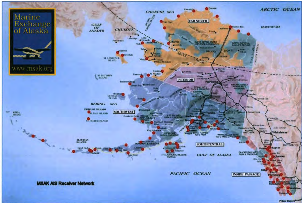
The red dots in the above graphic indicate the locations of the 120 Automatic Identification System (AIS) vessel tracking stations in Alaska built and operated by the Marine Exchange of Alaska to aid safe and environmentally sound maritime operations
