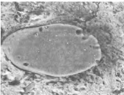
Figure 5. Scanning electron photomicrograph of a polished block of lignite from California. The minute (less than 1 micrometer) bright spots are rare grains of mercury selenide.
