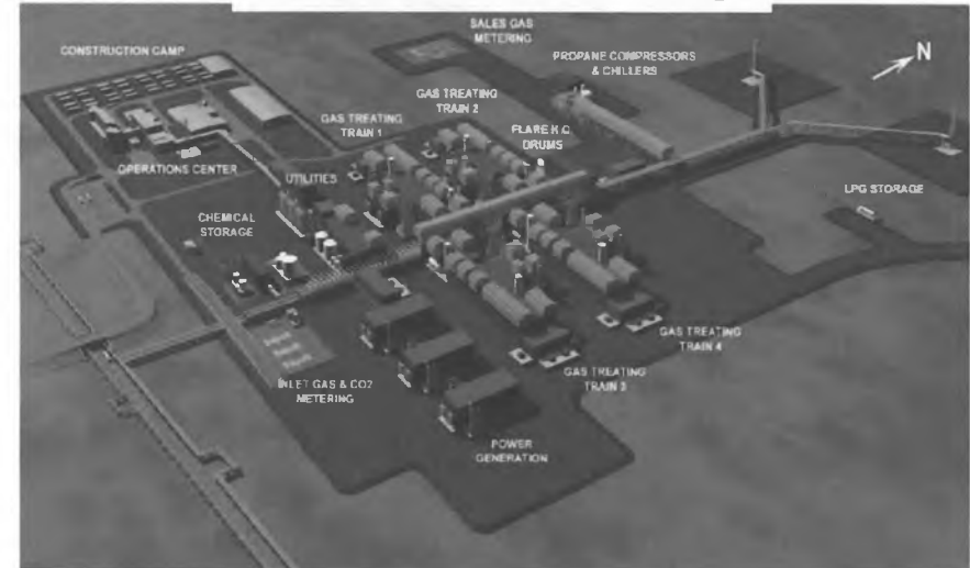
NS Gas Treatment Plant Design
