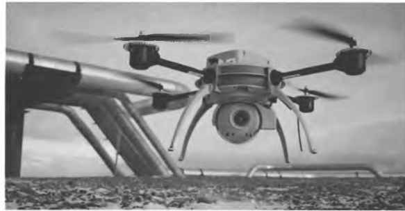
Figure 9: BP Utilized Aeryon Scout for Pipeline Inspections Jun 2013 17
