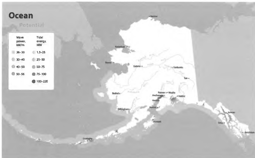
Total wave energy potential in Alaska is estimated to be 1,250 TWh/yr, more than 50 percent of the total potential found in the U.S. In addition to wave energy, Alaska is estimated to possess 90 percent of the tidal power in the U.S., or 109 TWh/yr.
