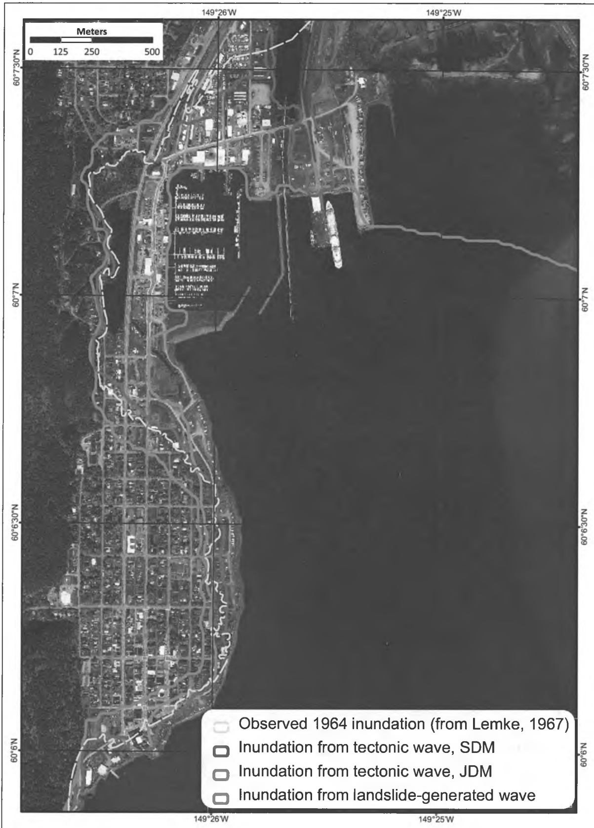
Figure 22. Observed 1964 inundation line (from Lemke, 1967) and calculated inundation lines from tectonic and landslide sources at Seward.
