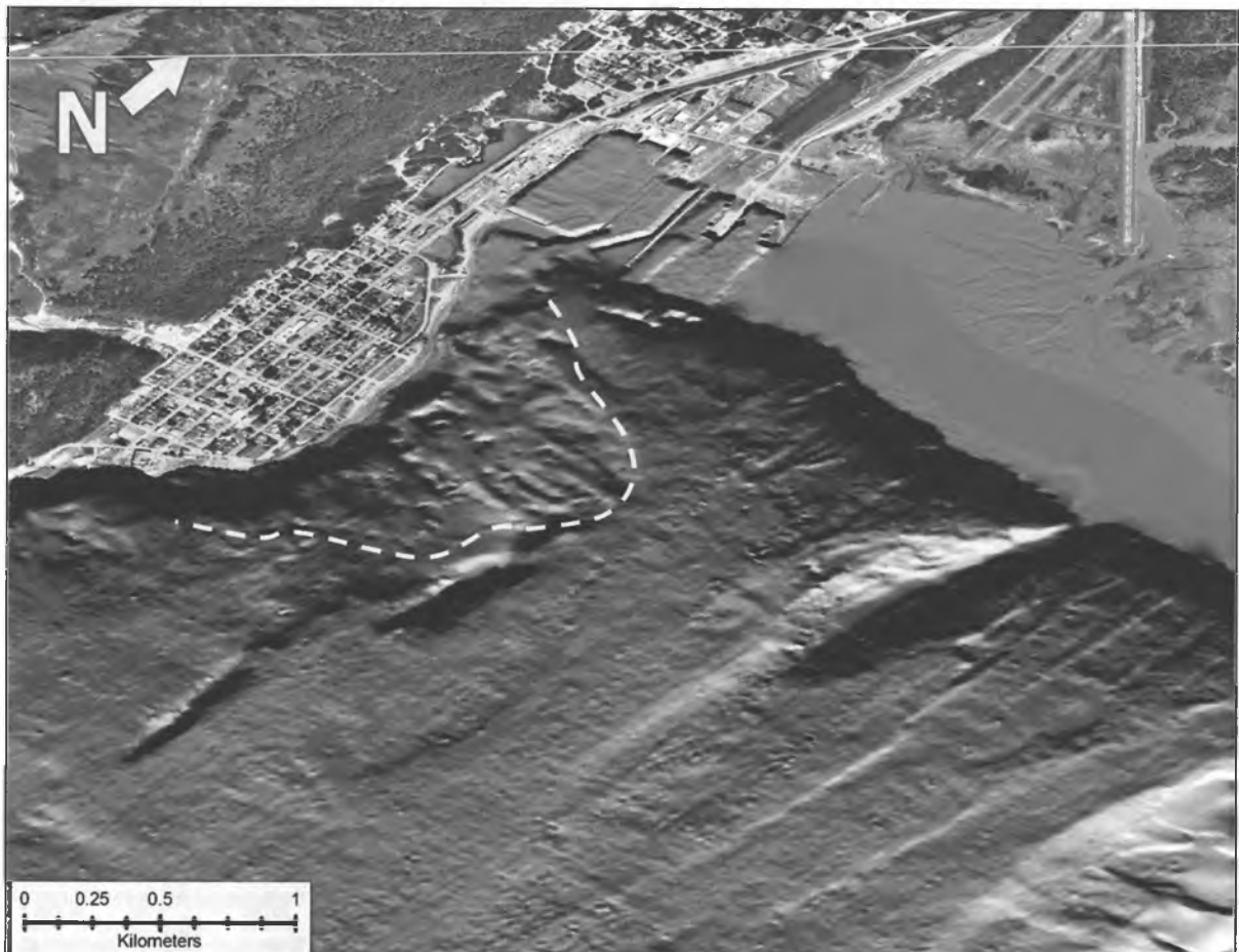
Figure 18. Oblique image of Seward downtown, with offshore shaded-relief bathymetry. Dashed white lines indicate the approximate margin of debris resulting from a submarine landslide that was triggered by the 1964 earthquake.
