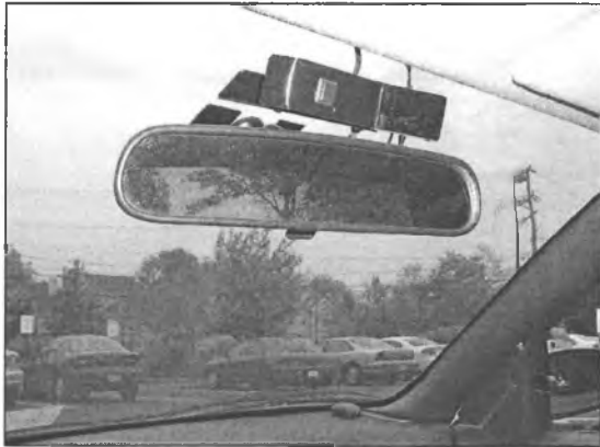
Figure 4. The incident push button box mounted above the rearview mirror. The portion on the right contains the driver face/left vehicle side camera hidden by a smoked plexiglass cover.
