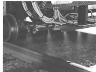
The herbicide AquaMaster is applied by a licensed contractor using a low-volume, low-pressure equipment to direct the herbicide only where it is intended.
