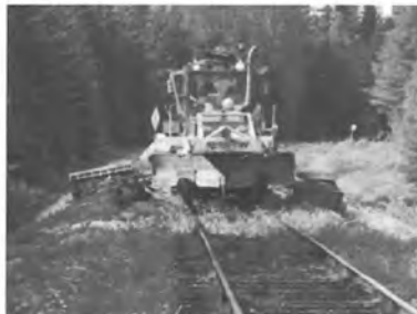
A brushcutter provides mechanical vegetation control along the track and shoulder. Vegetation in this area is more effectively controlled with herbicides.
