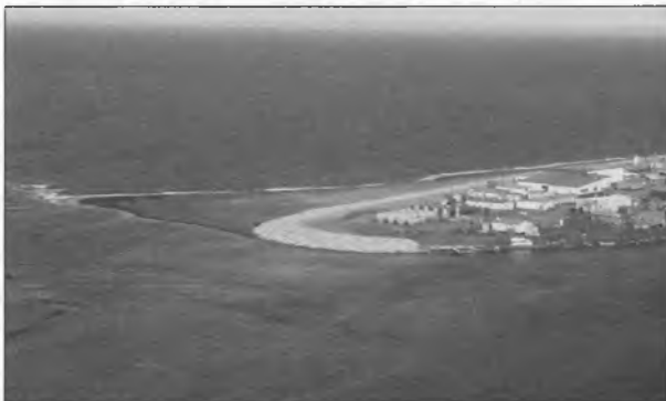
Figure 2. The village of Kivalina, northwestern Alaska. The engineered rock barrier is designed to help protect the town against coastal erosion.
