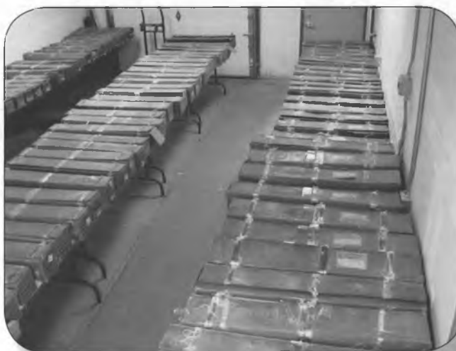
Figure 1: Several rows of temporary tables barely hold the 30- to 40-pound boxes of 5-inch core.
