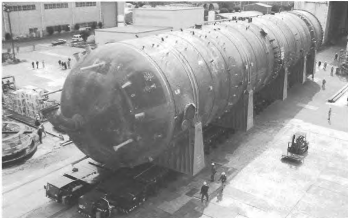
Figure 7-3: Transport of one 17,000 bbl/day Slurry-Phase FT Reactor [8]
