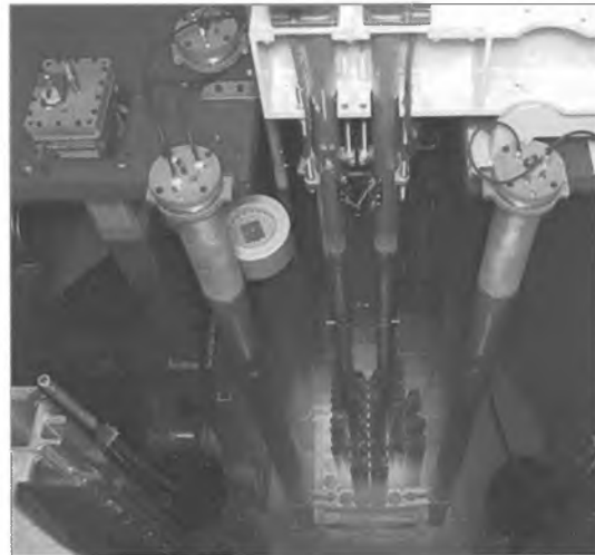
Figure 6. Core of a TRIGA research reactor, designed and constructed by General Atomics.
