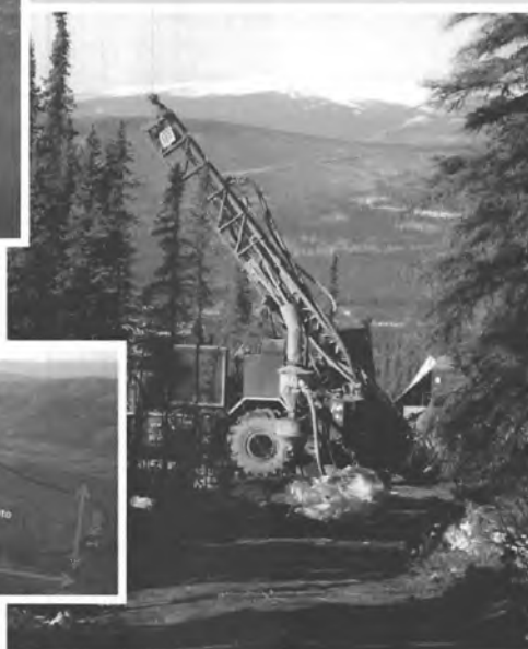
Reverse circulation drill rig on Money Knob
