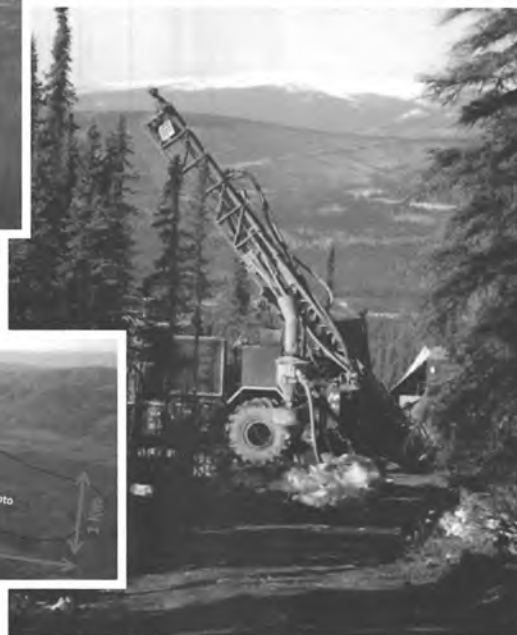
Reverse circulation drill rig on Money Knob
