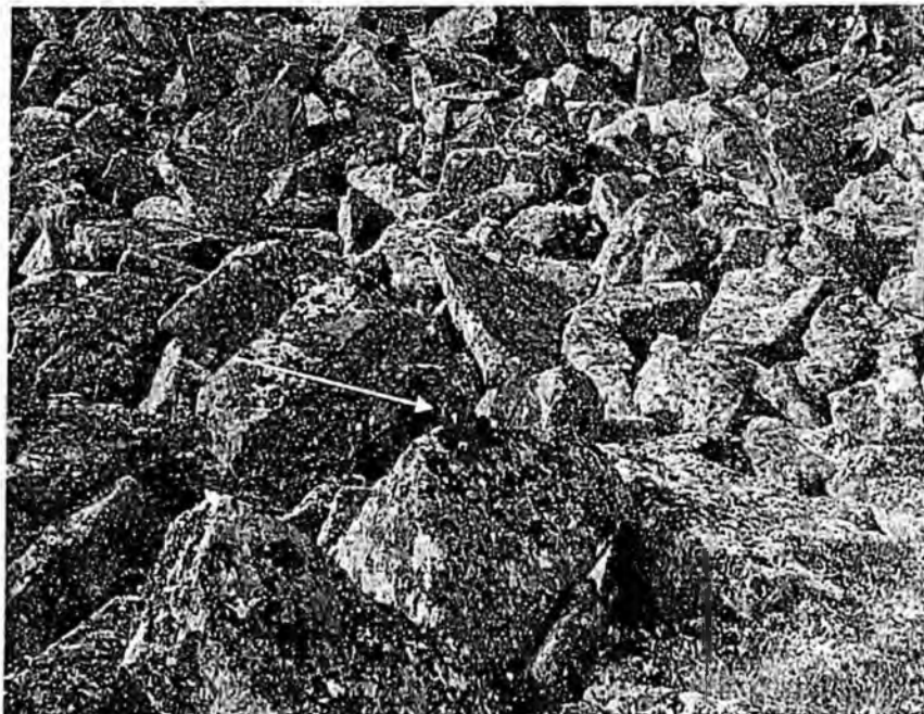
Figure 16 - Granite deposits on the top of Ear Mountain can be used for riprap. The arrow points to a glove.
