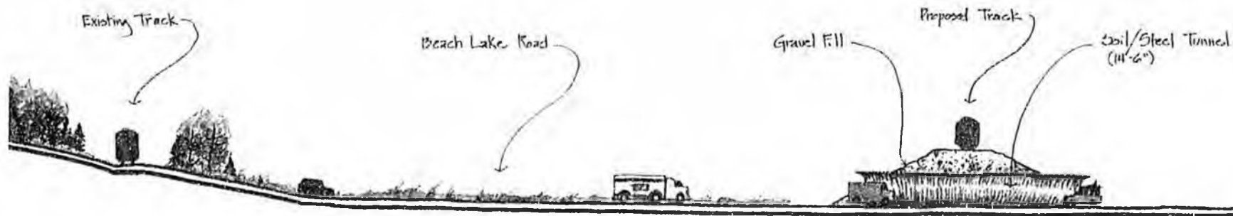
Section Through \phi Beach Lake Road Realignment
