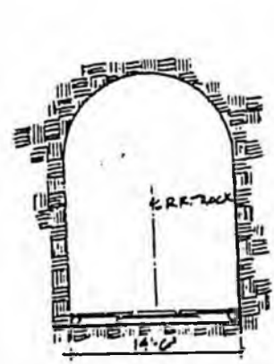
EXISTING RAILROAD SECTION
