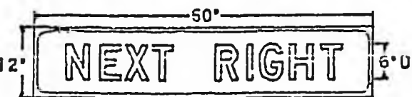
ALTERNATE SIGNS FOR ADVANCE SIGN PANELS
