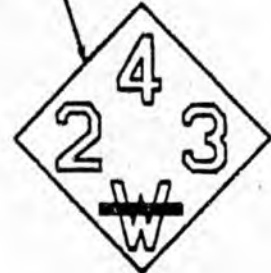
Fig. 3. For Use Where White Background is Used With Painted Numerals, or, For Use When Signal is in the Form of Sign or Placard
