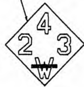
Fig. 3. For Use Where White Background is Used With Painted Numerals, or, For Use When Signal is in the Form of Sign or Placard
