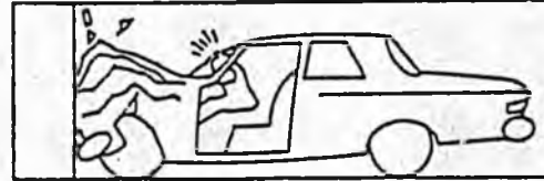
1/50 of a second after the car has stopped, the unbelted person slams into the dashboard or windshield. This is the human collision.
