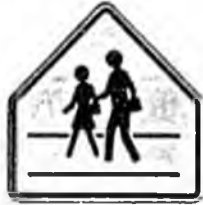
School Sign—similar to advance school sign but located at established school crossings.
