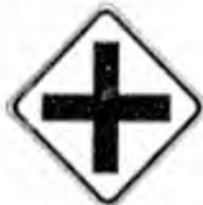
Crossroad. On through highway, warns of obscured crossroad intersection.
