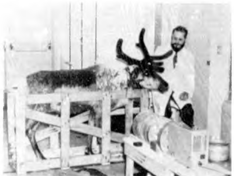
The photograph shows the portable scintillation counter being used to measure the radioisotope body burden of male reindeer "Pierre".
