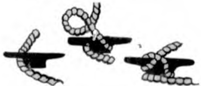
How To Make Fast To A Cleat
