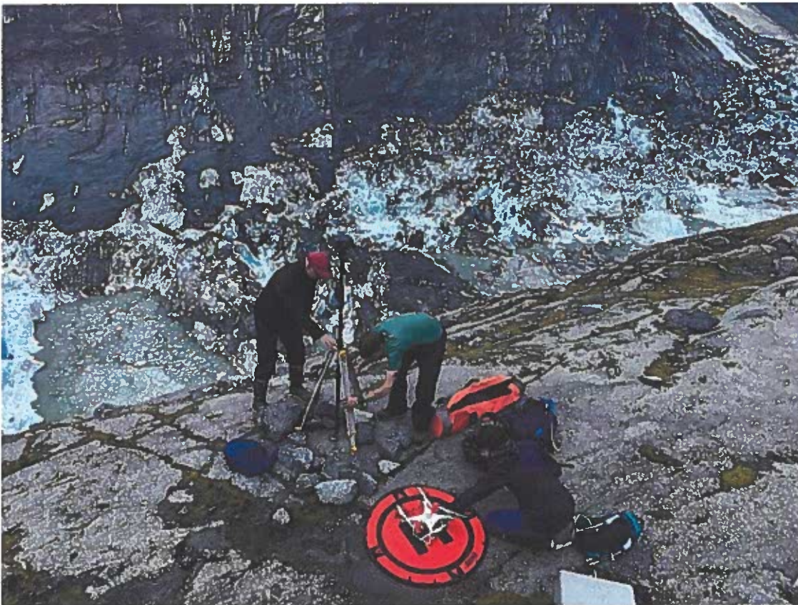
By doing repeated drone flights, researchers can build a 3D model to estimate the volume of water held in Suicide Basin. The basin is almost entirely empty after the flood on Saturday, Aug. 5, 2023 with just a few remaining pools of meltwater at the bottom (Anna Canny/KTOO)
