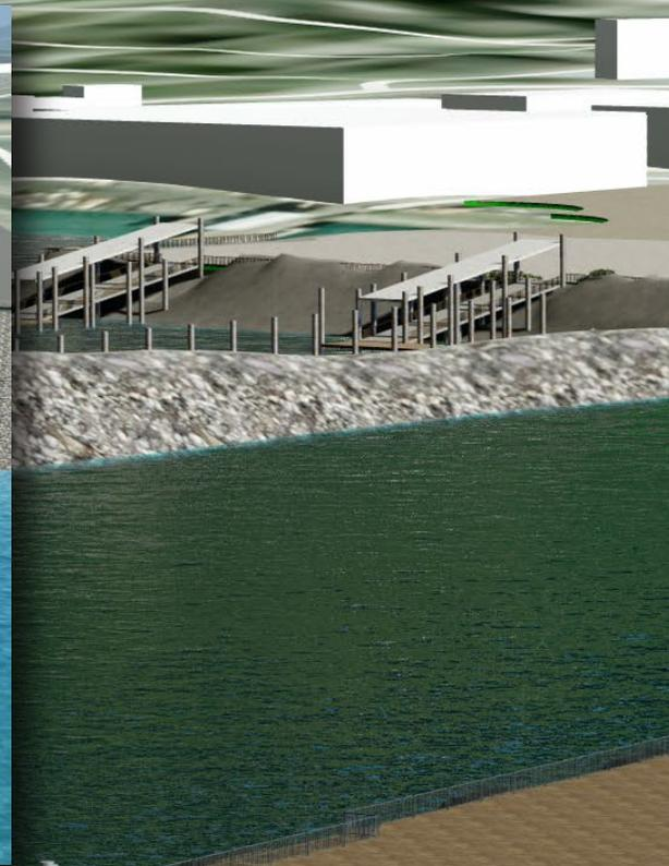
The floating double berth is 100 feet wide and 748 feet long. The 200-foot long split transfer span safely ushers cruise passengers and provisioning vehicles on and off the floating berth. For maintenance and to extend the life of the barge platform, the float is built in two sections specifically to be serviced in Seward's dry-dock facilities. The modernization of the pier includes a portable shore-power system.
