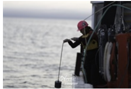
Sarah brings an acoustic transducer back onboard after communicating with an acoustic release. Credit: Brendan Smith/NPRB
