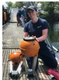
Sarah works to put up pop-up floats in Lake Washington to test them before deployment. Credit: NOAA/Heather Tabisola
