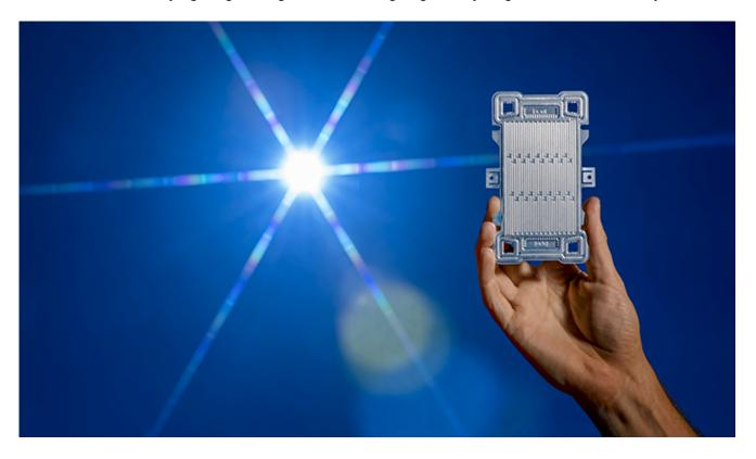
A component in a reverse fuel cell uses renewable power to knit together water and nitrogen to make ammonia.
