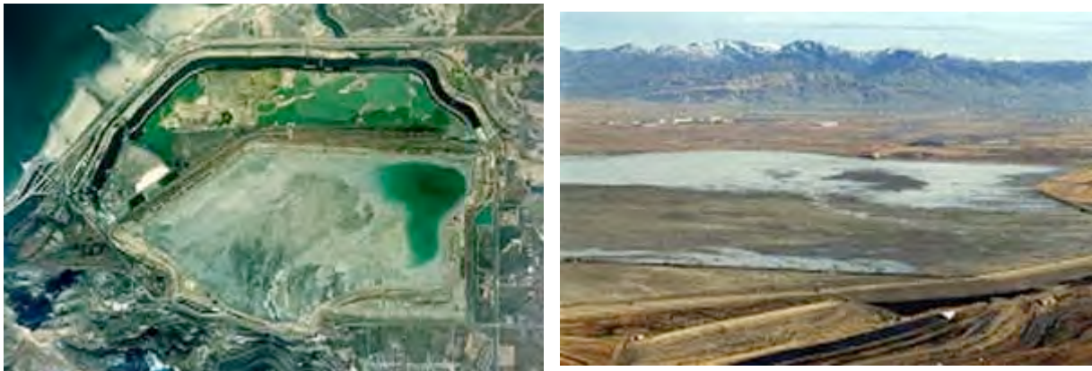
Figure 8. Kennecott Bingham Canyon Mine in Utah. (Left) Tailings impoundment (roughly 9,000 acres) with the Great Salt Lake at the top left. The pit is 0.75 miles deep, 2.5 miles wide, and covers 1,900 acres. (Right) Tailings are shown in the foreground (grey) with Salt Lake City in the background. Operations produced a 60 square-mile groundwater plume under valley to right, mostly from waste rock seepage. As of 2006, Kennecott had spent $370 million on cleanup and source control, and will be required to pump and treat aquifer water for at least the next 40 years. By 2009, 2.7 billion gallons of water will be treated annually to supply homes unable to use the aquifer.
